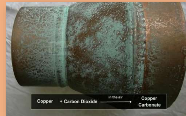
2) Green coating on copper
